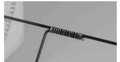
After the epoxy has set, remove the bearing once more. Insert the 1/32" wire of the wire assembly into the bearing. Attach the screw to the base from the rear and thread the nut onto it. Do not tighten. Feed the cotter pin end of the wire assembly into the scale hole. Move it back and feed the pin into the screw. Move it back as far as it will go. Mark the 1/32" wire about 1/16" in front of the bearing. Then pull the shaft forward as far as it will go.
