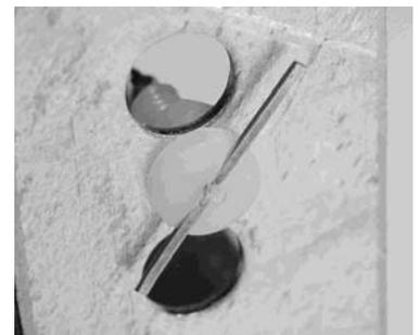
Push the cotter pin back as far as possible. Rotate the pin until the fingers are aligned with the screw slot. Bend the fingers over into the slot on both sides. You can cut off the ends, but leave some extending from the screw head.
