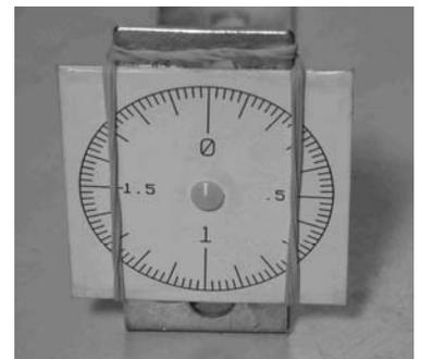
Put the bearing through the scale and insert it into the 1/8" hole in the base. Align the board square with the base and mark the base along the top and bottom of the board. Remove the scale and apply some epoxy between the lines on the base, keeping it away from the bearing hole. Reattach the scale, with the bearing in it and the base. Align the scale to the base and hold in place with some rubber bands as in the photo.
